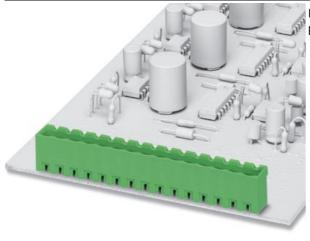
Header, nominal current: 12 A, rated voltage: 200 V, pitch: 5.08 mm, no. of positions: 2, mounting: Press in
